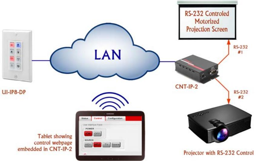
Use UI-IP8-DP with add-on CNT-IP-2 for control of RS-232 Devices
