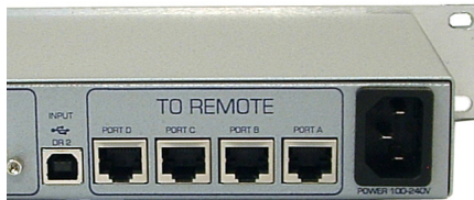
Close-up of Sender UTP Connections to the Remote Unit
