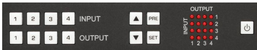
Figure 16 – Control buttons on the front panel
