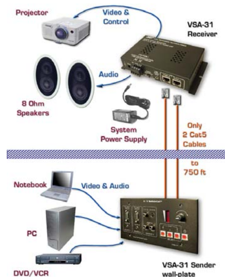
The Basic VSA-31 Block Diagram
